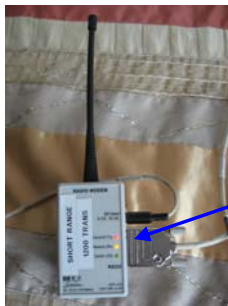
Lights come on for 2-3 seconds when power applied
